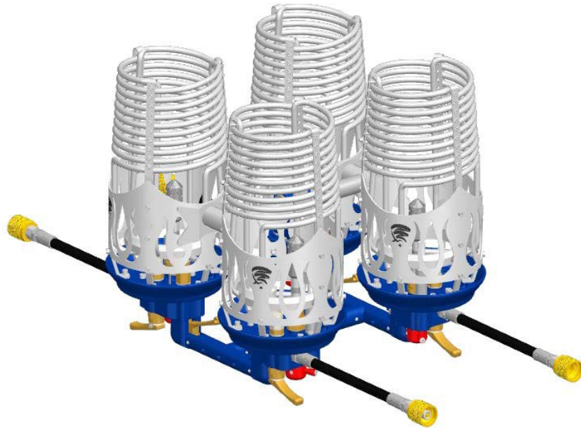
Figure 7. Quadruple burner general view
